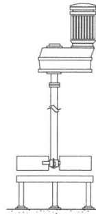
B. Submerged aerator
